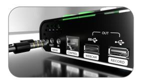
Connect the microphone to mini-pro's Audio IN port and connect the speaker or earphone to Audio OUT port.
