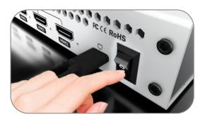
Turn on the Power button on the rear panel, the device will enter to the boot interface within 10S.
