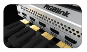
Connect PC,laptop,camera or DVD to mini-pro's HDMI IN port via HDMI cable.
