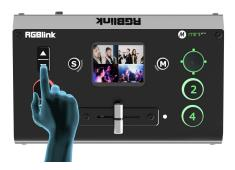
When the touch screen is in the main interface/ preview interface/Shortcut interface, the PGM audio volume can be adjusted by the toggle.
