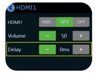
If the sound and the video are not synchronous, increase or reduce the Delay value under AFV.(External and HDMI input audio support delay up to 160ms)
