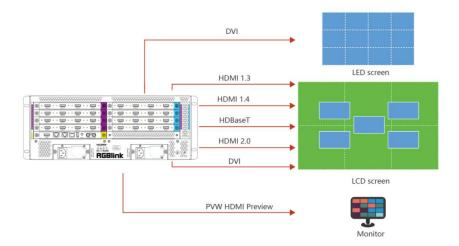
Q16pro Series supports SDI,DVI,HDMI,HDBaseT and other optional output modules. Connect Q16pro with monitors.
