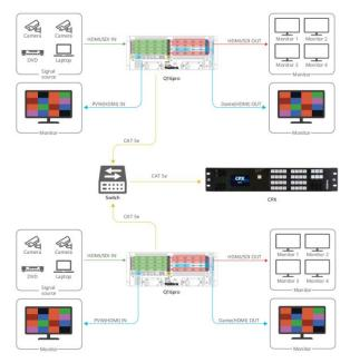
After successful connection, power on Q16pro and CPX. (Use the standard 12V power adapter to connect CPX and power socket in order to boot up CPX.) User should firstly choose Q16pro as the controlled device.
