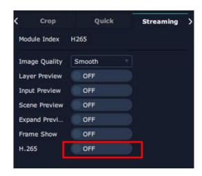
Note: H.265 is the master switch. If the user turns on H.264 first, it cannot be set successfully.
