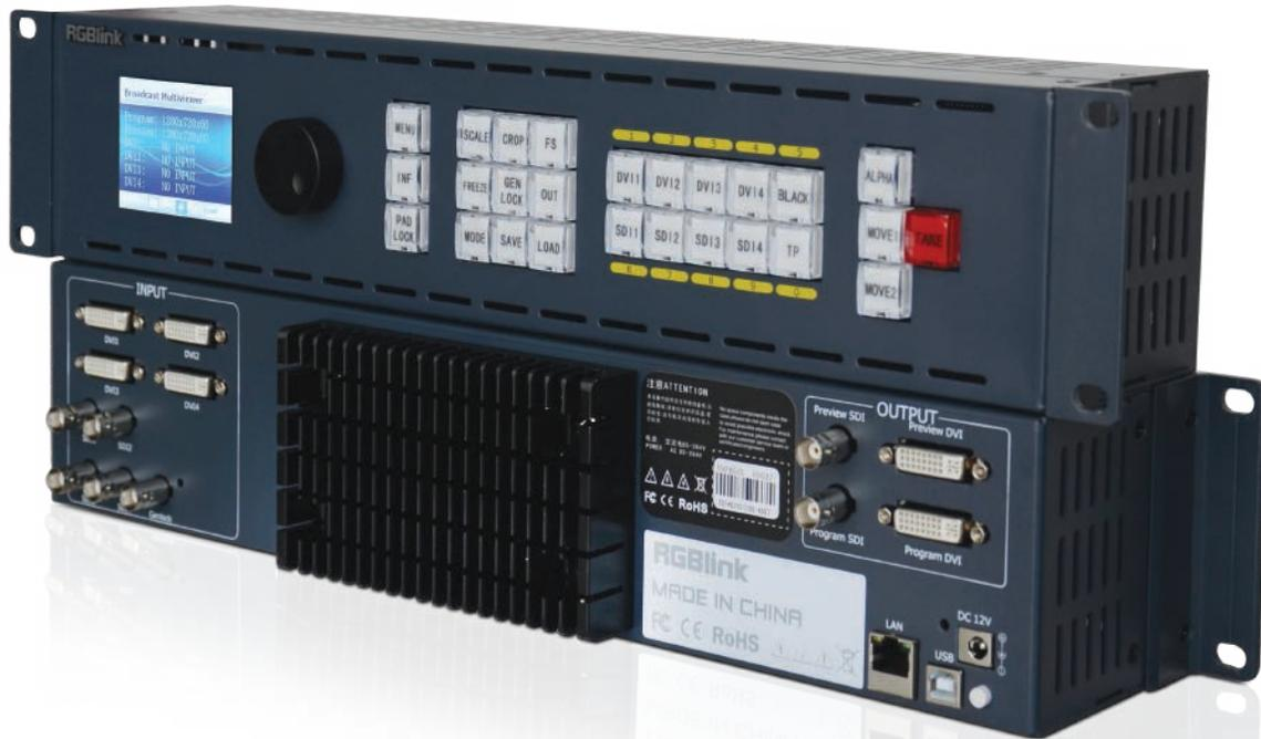
MVP8043 is a eight input professional Multi-viewer for broadcast applications or video wall control switching. Entirely solid-state, with MVP8043 there is a convenient ten window multi-view available via the Preview output for immediate viewing of available sources along with both the selected Preview and Program. MVP8043 features eight inputs – 4 SDI (up to 3G) as well as 4 DVI inputs. The Preview output is available with both SDI and DVI signals, as is the Program output.
